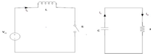
Fig. 2: ON Mode Circuit
