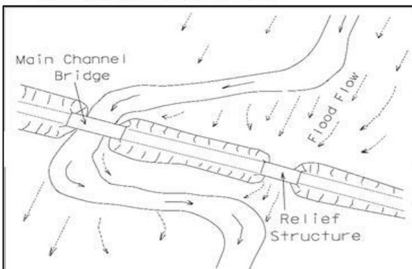
Fig. 2: Highway Stream Crossing at A Bend
