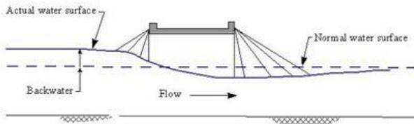
Fig. 1: Backwater at A Stream Crossing
