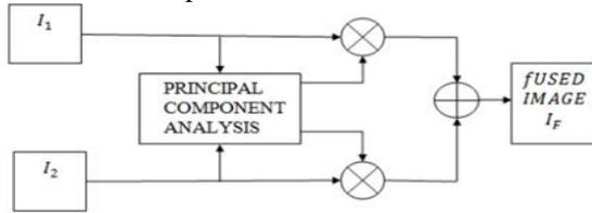
Fig. 2 Information flow diagram employing PCA<sup>[4]</sup>
