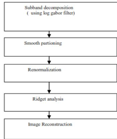
Fig. 12: Flow Chart of the Proposed Method<sup>[5]</sup>
