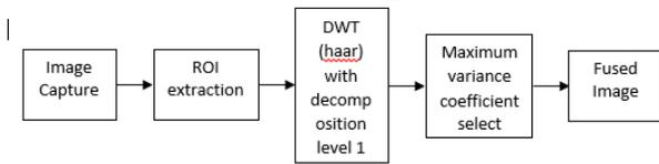
Fig. 8: Multispectral palm image fusion system.
