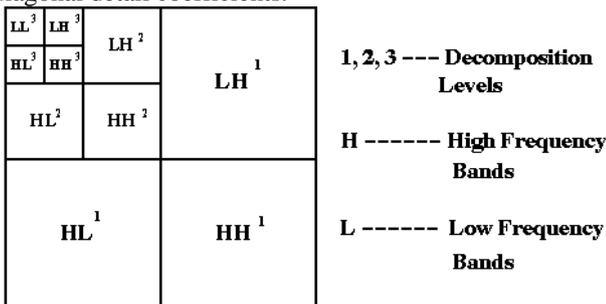
Fig. 4: DWT decomposition image
