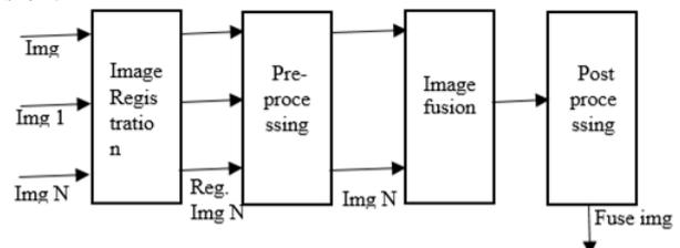
Fig. 1: Pixel level image fusion.
