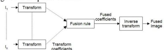
Fig. 9: Generic method for transform based fusion<sup>[3]</sup>
