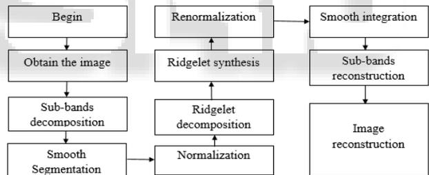
Fig. 6: Flow diagram of Curvelet transforms
