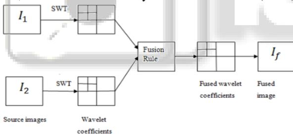
Fig. 11: Information flow diagram in image fusion scheme employing SWT<sup>[4]</sup>
