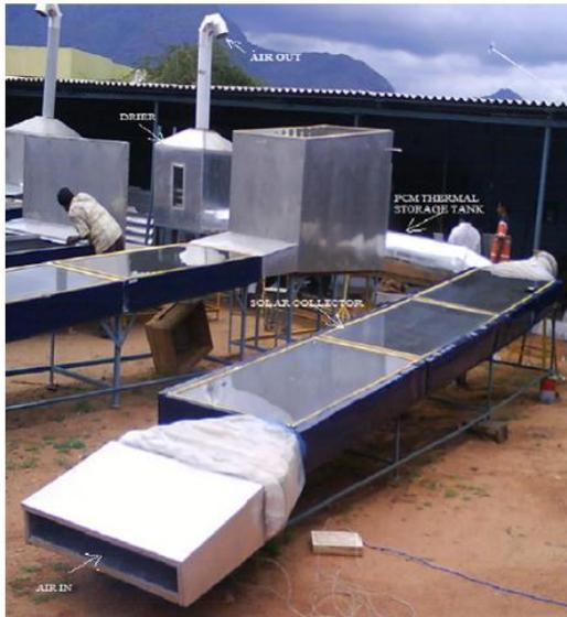
Fig. 3: Experimental Setup of S.Esukkimathu[1]
