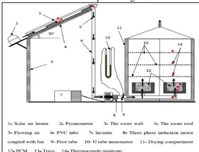
Fig. 4: S.M. Shalby, M.A. Bek Experimentation arrangement[2]
