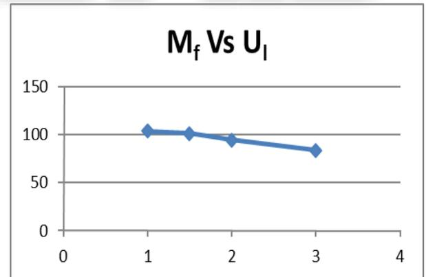
Fig. 4: Graph 2. Mass flow rate (M<sub>f</sub>) vs. overall Heat loss coefficient (U<sub>l</sub>)
