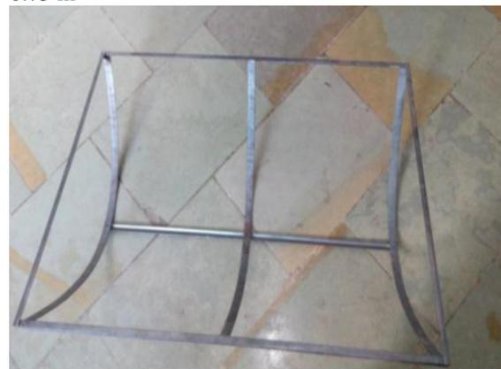
Fig .1: Parabolic Trough
