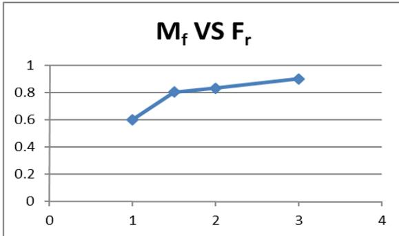
Fig. 5: Graph 2. Mass flow rate ( $M_f$ ) vs. Heat removal factor ( $Fr$ ).
