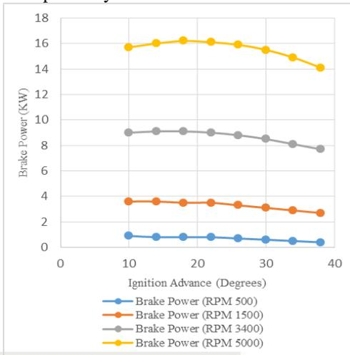
Fig. 6: Graph 4: Brake Power Vs Ignition Advance
