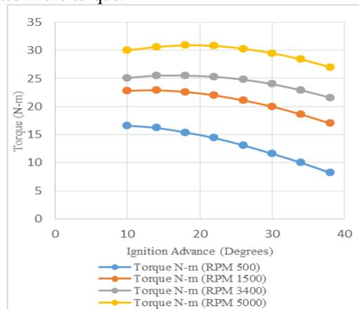
Fig. 4: Graph 2: Torque Vs Ignition Advance
