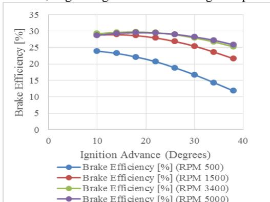
Fig. 3: Graph 1: Brake Efficiency Vs Ignition Advance
