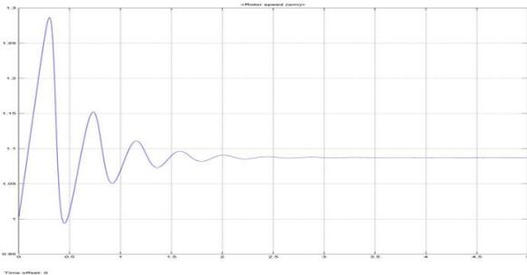
Fig. 7: Rotor speed of SEIG
