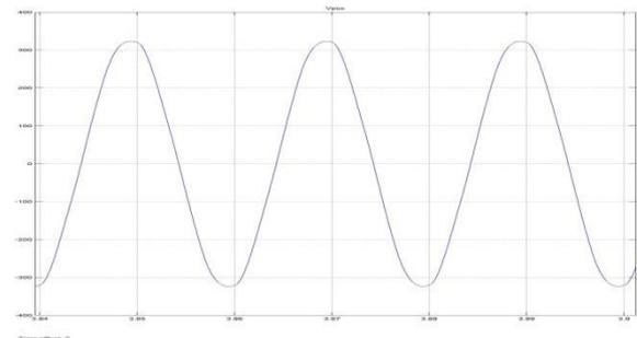
Fig. 12: Smoother inverted output line to line voltage waveform
