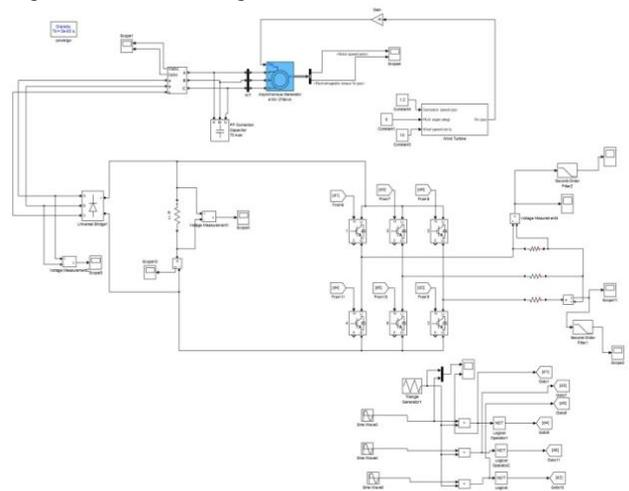
Fig. 4: Simulink model of SEIG fed with wind turbine
