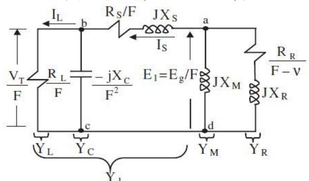
Fig. 2: Per phase equivalent circuit of SEIG
