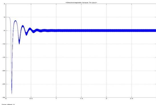
Fig. 8: Electromagnetic torque of SEIG
