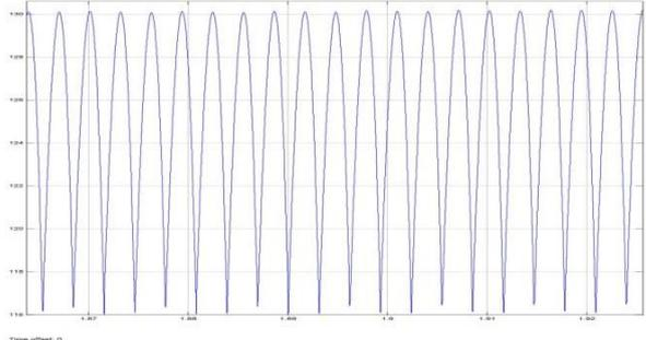
Fig. 10: Rectified d.c current waveform
