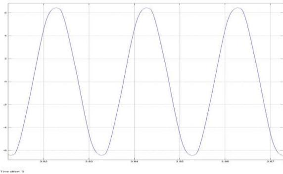
Fig. 14: Smoothen inverted output line to line current waveform
