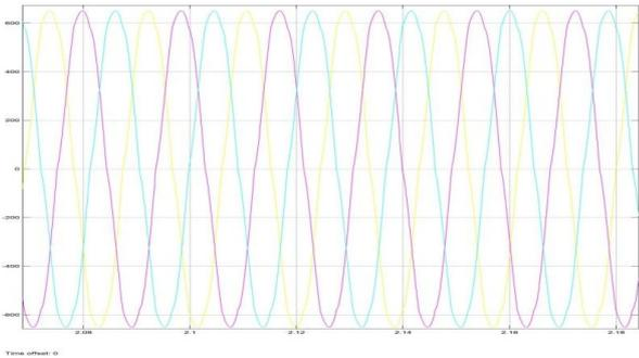
Fig. 5: Generated output voltage of SEIG
