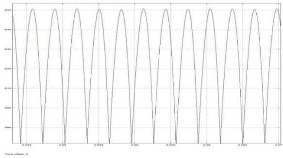
Fig. 9: Rectified d.c voltage waveform
