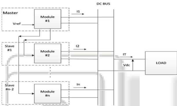
Fig. 2: Schematic diagram of Master Slave Control
