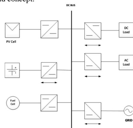
Fig. 1: Generic topology of a dc micro grid
