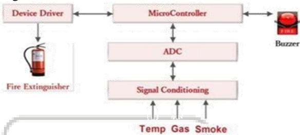
Fig. 2: Basic System Block Diagram
