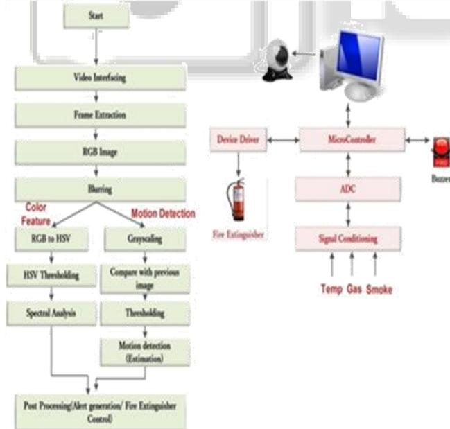
Fig. 3: Basic Block Diagram of Proposed System
