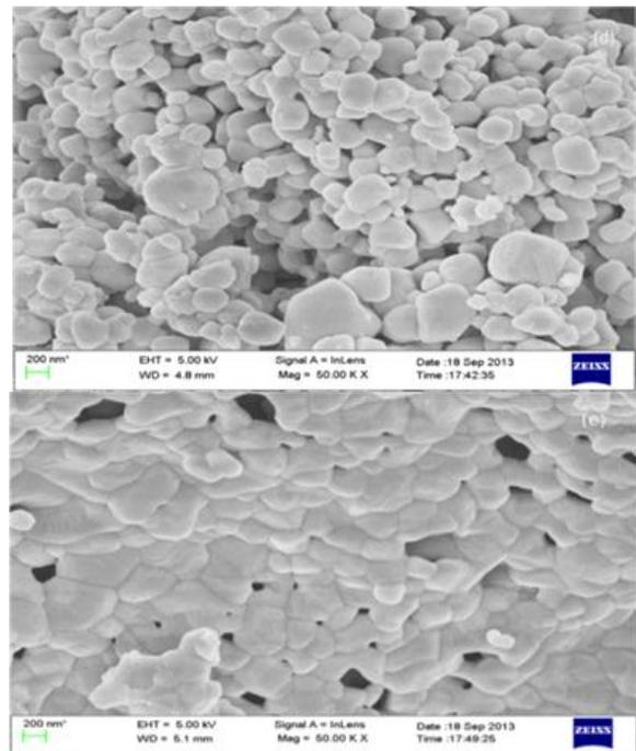
Fig. 2 (a): FESEM micrograph for pure powders of MCZF, (b): BaTiO<sub>3</sub> and (c): MBT1 nano composite, (d): MBT2 and (e): MBT3 nano composites
