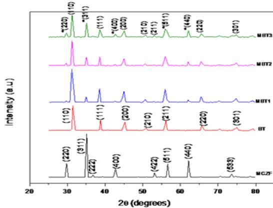
Fig.1 XRD Pattern for pure nano powders of Mg<sub>0.25</sub>Cu<sub>0.25</sub>Zn<sub>0.5</sub>Fe<sub>2</sub>O<sub>4</sub> (MCZF) and BaTiO<sub>3</sub> (BT) and MBT1, MBT2, MBT3 composites. Asterisk (\*) indicates ferrite phase.
