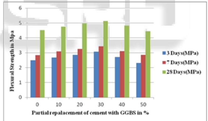
Fig. 9: Variation of Flexural strength of M20 Grade Concrete
