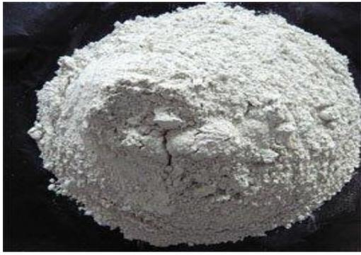
Fig. 1: Ground Granulated Blast furnace Slag
