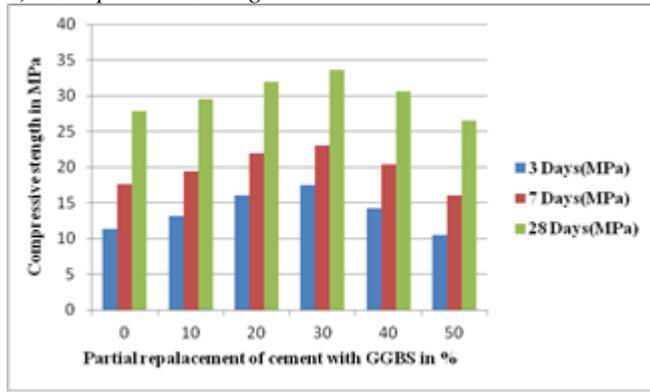
Fig. 5: Variation of Compressive strength of M20 Grade Concrete
