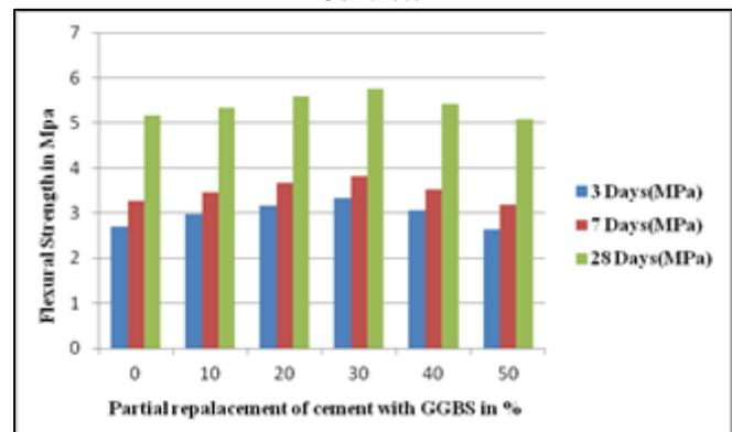
Fig. 10: Variation of Flexural strength of M30 Grade Concrete
