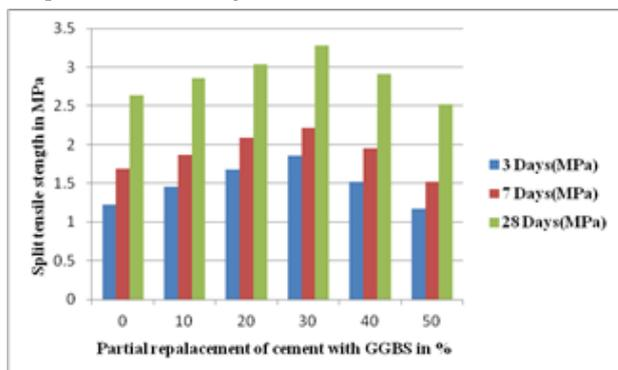
Fig. 7: Variation of Split tensile strength of M20 Grade Concrete
