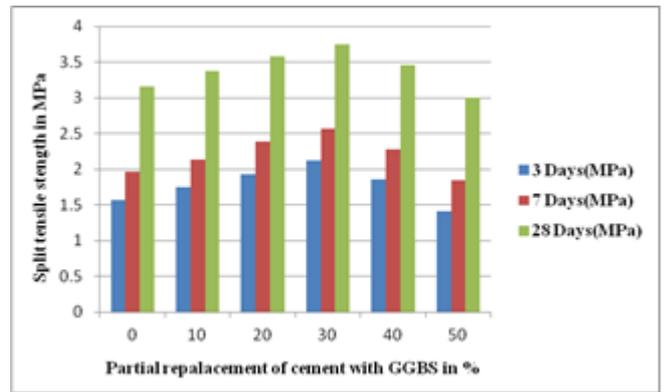
Fig. 8: Variation of Split tensile strength of M30 Grade Concrete
