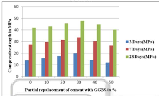
Fig. 6: Variation of Compressive strength of M30 Grade Concrete
