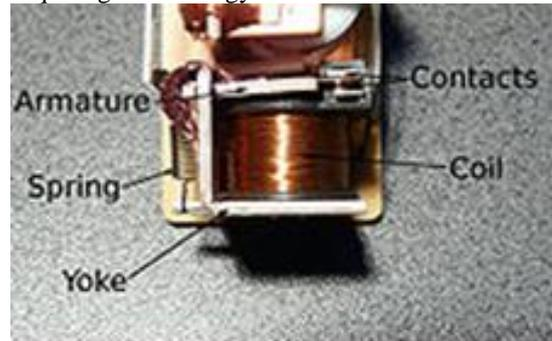
Fig. 5: Relay Coil
