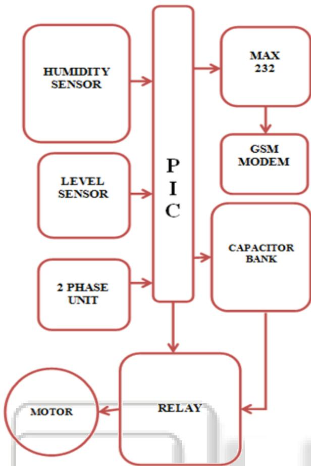
Fig. 7: Schematic Diagram of proposed system
