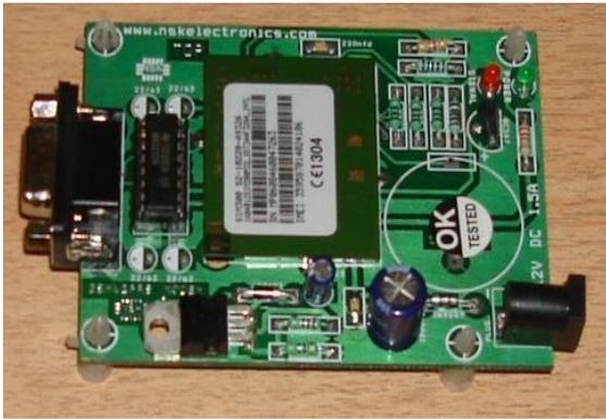
Fig. 3: GSM Modem
