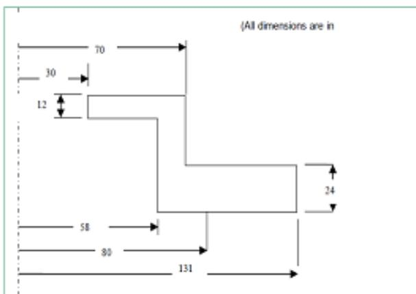
Fig. 2: Dimensions of disk brake rotor
