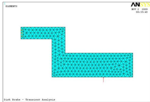
Fig. 3: Meshed model of disk brake rotor
