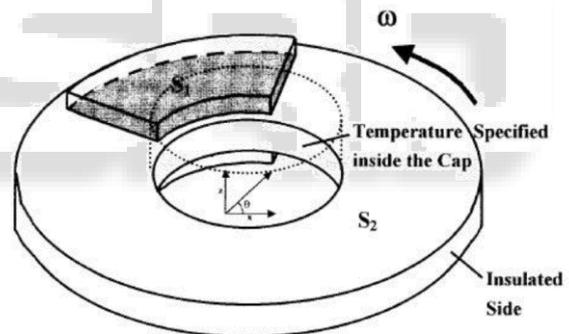
Fig. 4: Disk brake for thermal analysis
