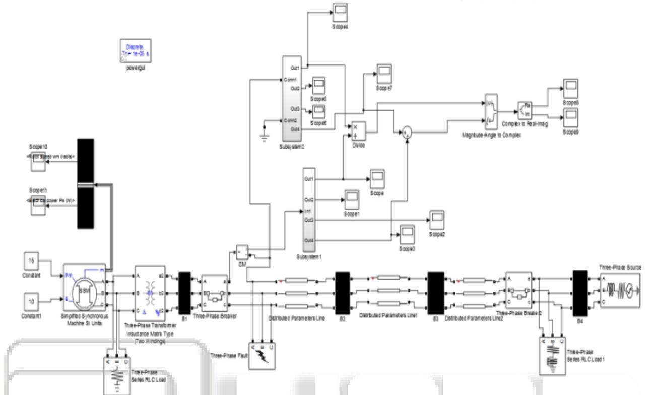
Fig. 2: Simulation model of distance relay.
