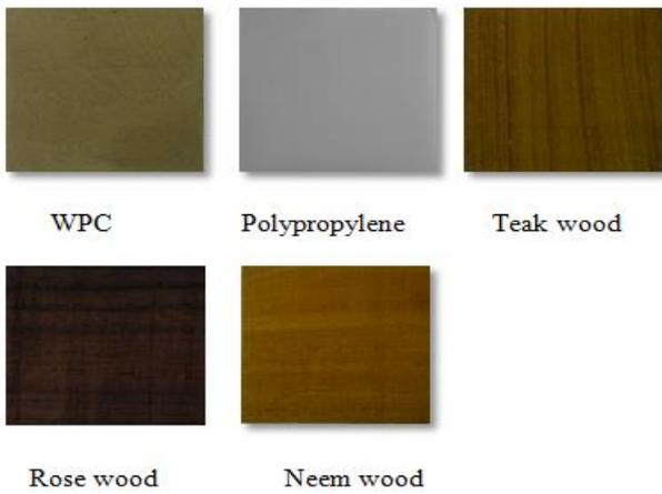
Fig. 9: Specimens used for heat resisting test
