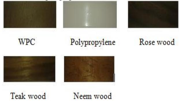
Fig. 7: Specimens used for moisture content test
