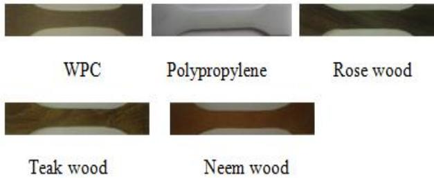
Fig. 4: Specimens used for tensile test
