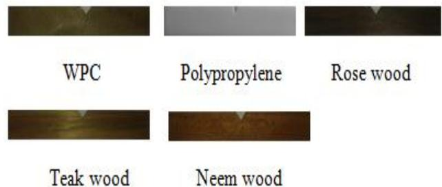
Fig. 3: Specimens used for izod impact test
