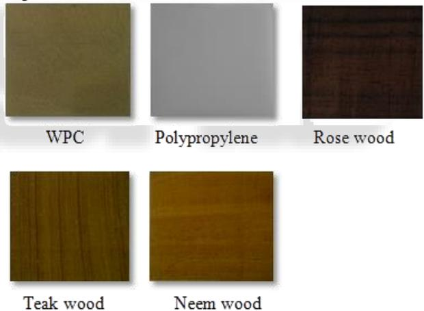
Fig. 8: Specimens used for water absorption test
