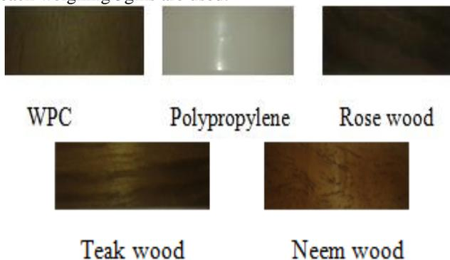
Fig. 6: Specimens used for specific gravity test
