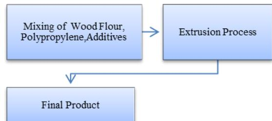
Fig. 1: A typical production flowchart of wood plastic composite
