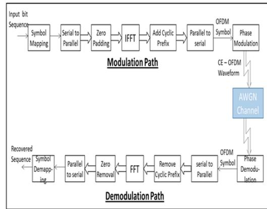
Fig. 1: Block diagram of CE-OFDM system
