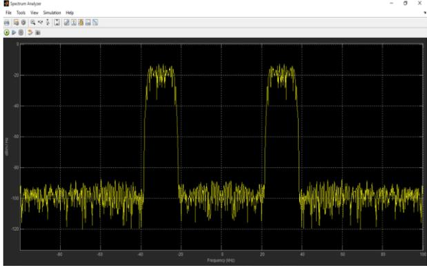
Fig. 7: Standard OFDM Spectrum
