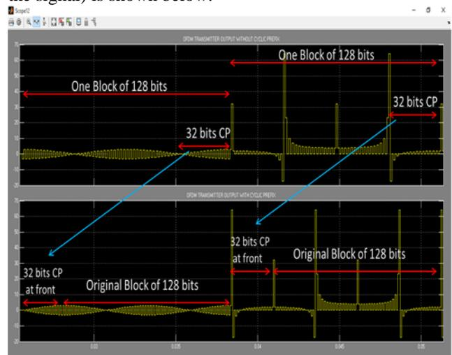
Fig. 5: Cyclic prefix added binary signal
