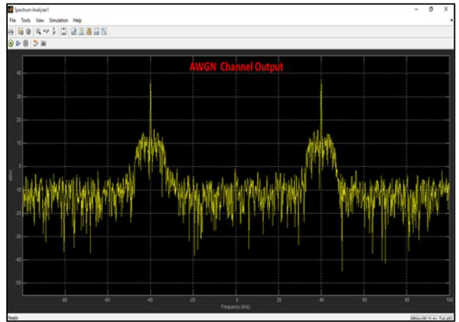
Fig. 9: Received CE-OFDM Spectrum
