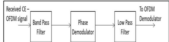
Fig. 2: Band pass to base band conversion
