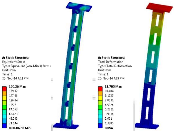
Fig. 5: Load Case – III: ANSYS results for Equivalent stress & Total deformation
