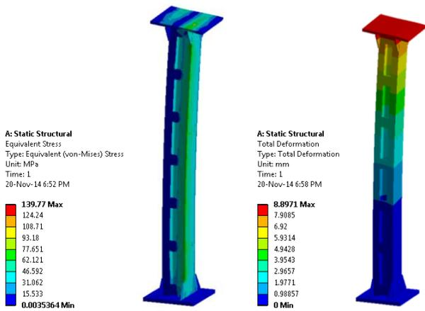
Fig. 4: Load Case – II: ANSYS results for Equivalent stress & Total deformation
