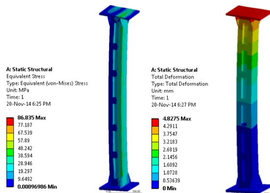
Fig. 3: Load Case - I: ANSYS results for Equivalent stress & Total deformation
