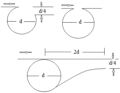
Fig. 2.3: Various type of the vortex tube sand traps tested by Parshall
