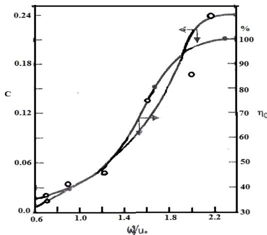
Fig. 2.2: Garde's curve Variation of  $\eta_0$  and C with  $\omega_0/u$
