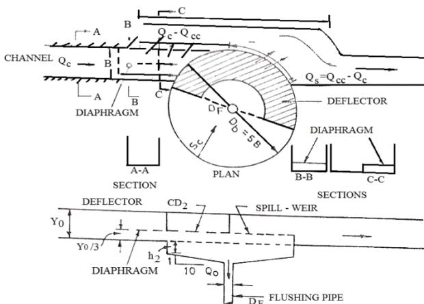
Fig. 2.5: Vortex settling basin
