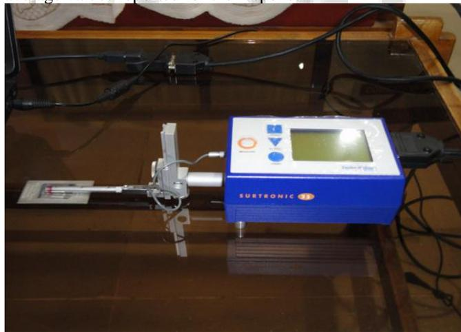
Fig. 5: Surface roughness tester, Taylor Hobson (Surtronic 25)
