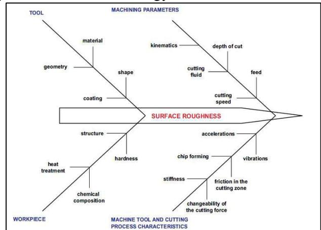
Fig. 1: Parameters affects the surface roughness
