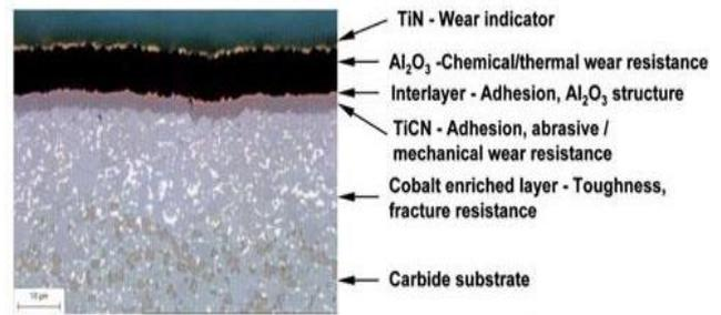
Fig. 4: Carbide Tool Structure
