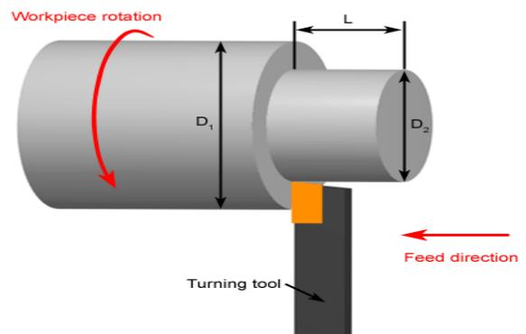
Fig. 2: turning operation
