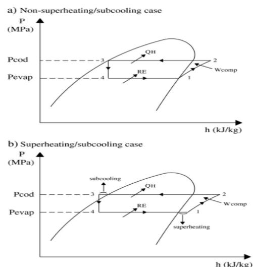
Fig: (a) non-superheating/subcooling
