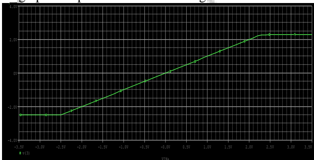
Fig. 6: Input common mode range of OPAMP
