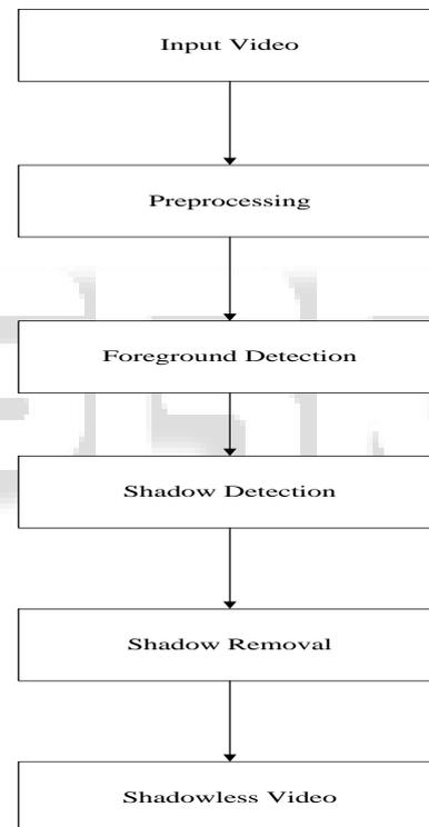
Fig 1 : phases of shadow detection and removal system
