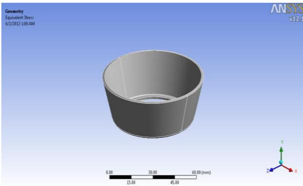
Fig. 3: Geometry of cage
