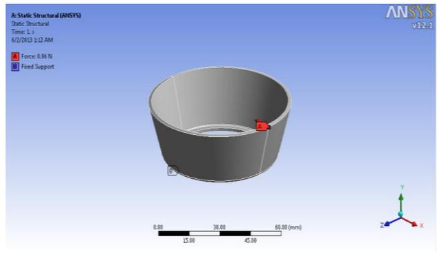
Fig. 5: Load applied on cage
