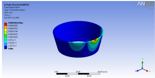
Fig. 6: Total deformation of cage
