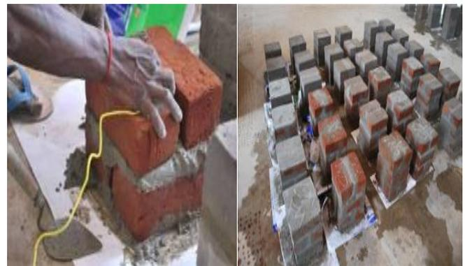
Fig. 1: Casting of Clay Brick Prisms
