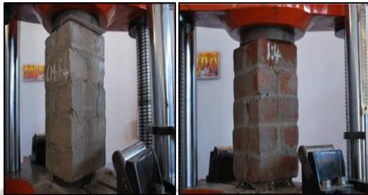
Fig. 3: Compressive Strength Test for Brick Masonry Prism
