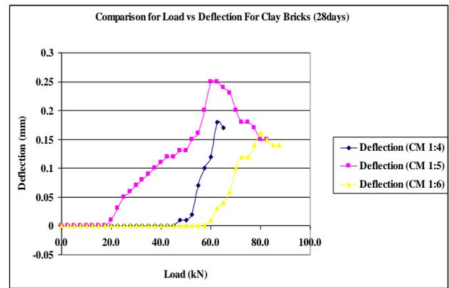
Fig. 8: Load vs. Deflection Curve Clay Brick Masonry Prism (28days)
