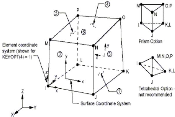
Fig. 15: Solid 185, 3D solid element type
