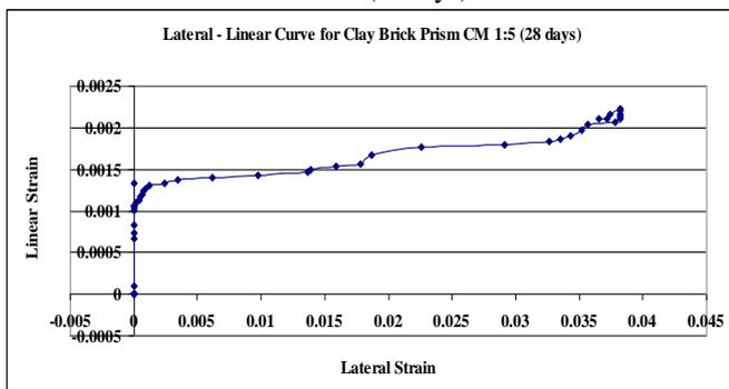
Fig. 13: Lateral vs. Linear Strain for Clay Brick Prism CM 1:5 (28days)
