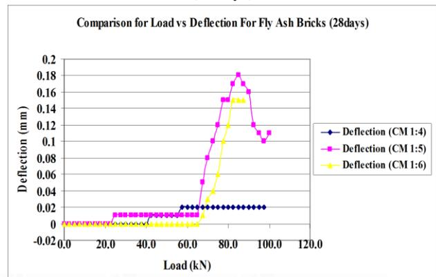
Fig. 9: Load vs. Deflection Curve Fly Ash Brick Masonry Prism (28days)
