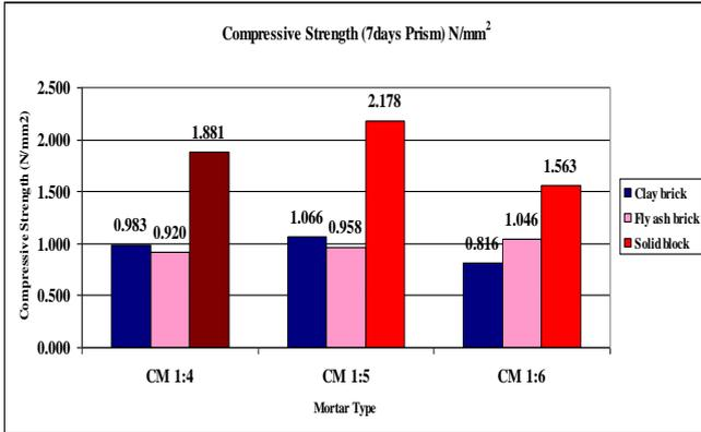
Fig. 6: Compression Strength for Bricks
