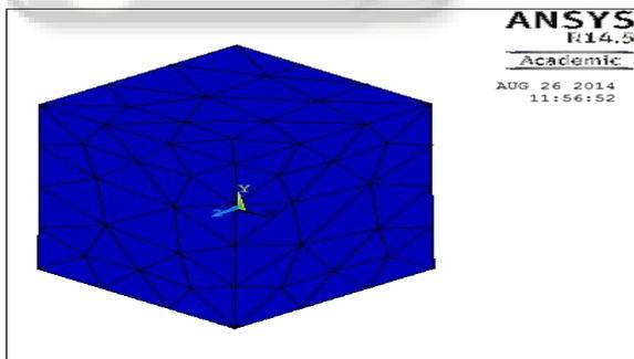
Fig. 16: Macro level modeling of brick masonry prism
