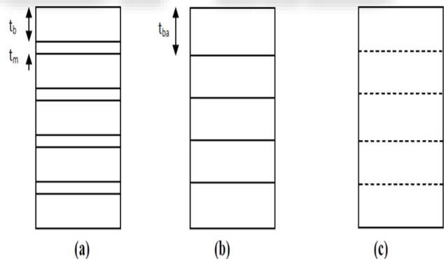
Fig 14 – (a) Micro level modelling (b) Meso level modelling(c) Macro level modelling
