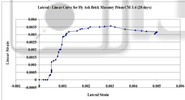
Fig. 12: Lateral vs. Linear Strain for Fly Ash Brick Prism CM 1:4 (28days)
