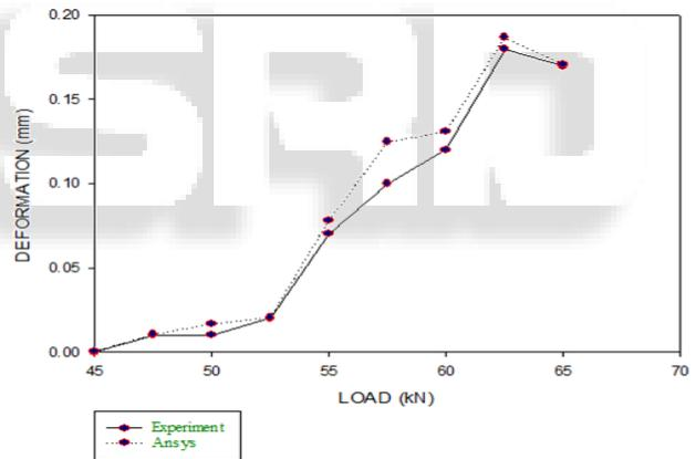
Fig. 19: Load vs. Deflection Curve Fly Ash Brick Masonry Prism (28days)
