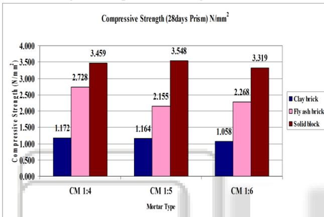
Fig. 7: Compression Strength for Bricks
