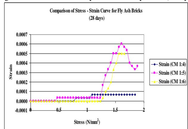
Fig. 11: Stress Strain for Fly Ash Brick Masonry Prism (28days)
