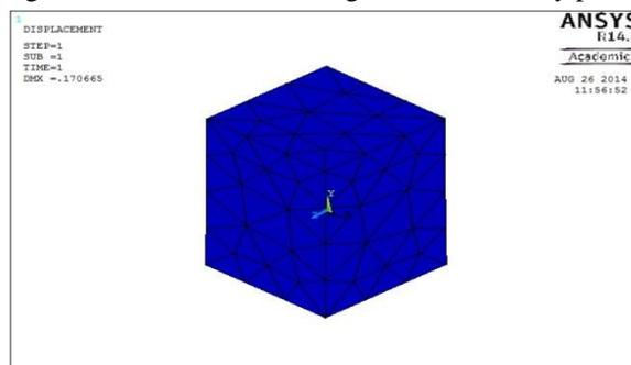
Fig. 17: Deflection of Clay Brick Masonry Prism CM 1:4 (28days)
