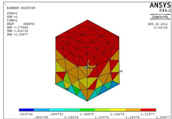
Fig. 18: von mises stress of Clay Brick Masonry Prism CM 1:4 (28days)
