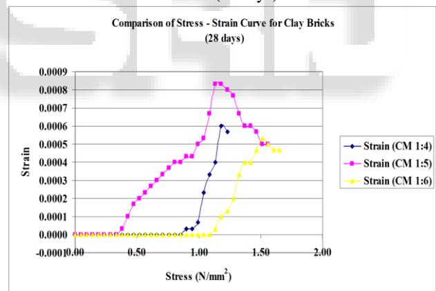
Fig. 10: Stress Strain for Clay Brick Masonry Prism (28days)
