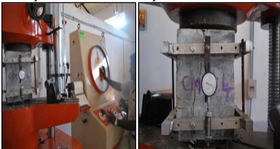
Fig. 4: Test set up for Young's Modulus of Elasticity
