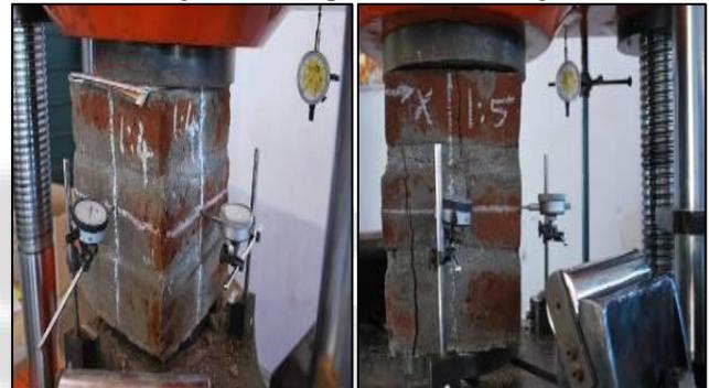
Fig. 5: Test set up for Poisson's Ratio (Clay Brick Prism)
