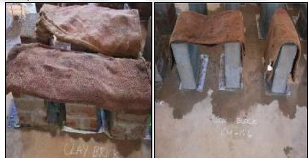
Fig. 2: Curing of Brick Prisms
