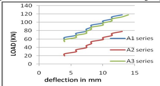
Fig. 4: Load deflection behavior of beams of group B
