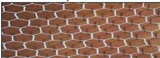
Fig. 1: Hexagonal wire mesh
