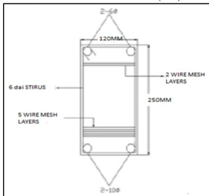
Cross section of beam (A3)
