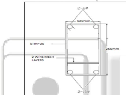
Cross section of beam (A1)
