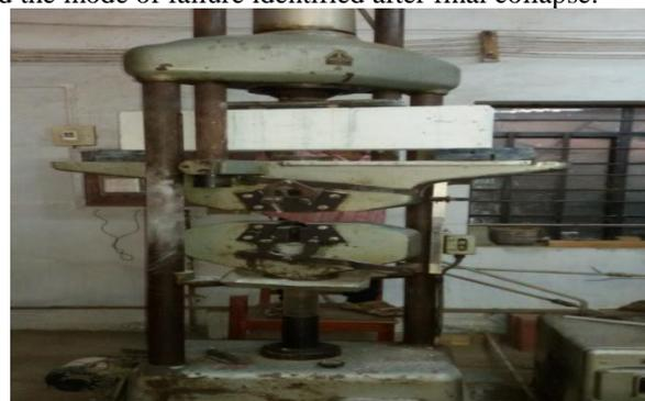
Fig. 2: Test Setup for beam
