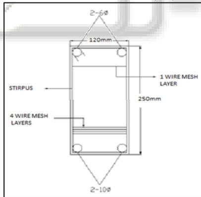
Cross section of beam (A2)
