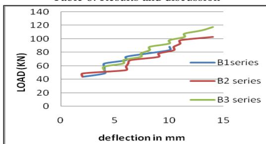
Fig. 3: Load deflection behaviour of beams of group A
