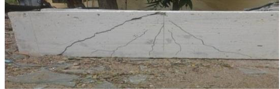
Fig. 6: Shear Failure observed in beams
