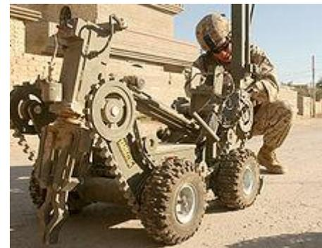
A U.S. Marine Corps technician prepares to use a telerobot to detonate a buried improvised explosive device
