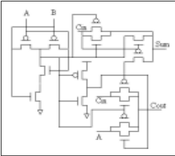
Fig. 3 14T Full Adder Cell
