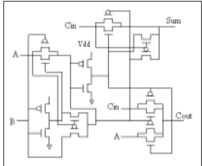
Fig.1 Transmission Function Adder
