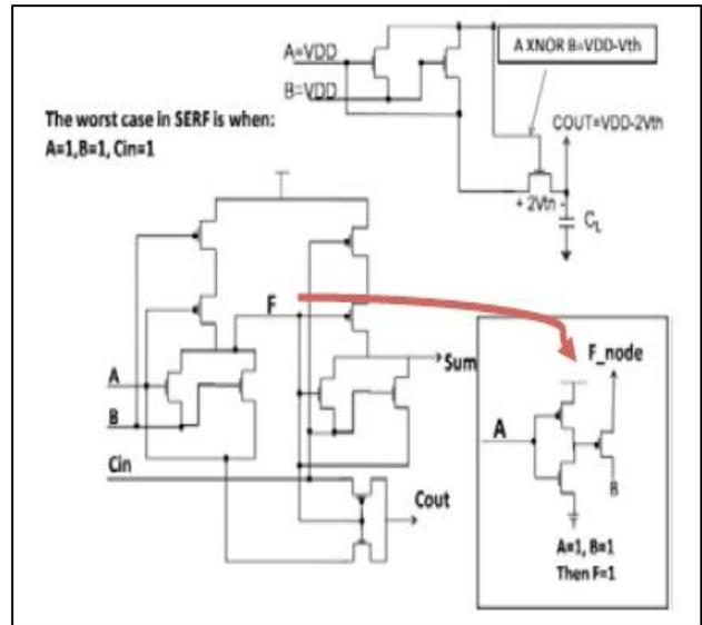
Fig.5 Modified SERF ADDER CELL
