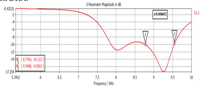
Fig.3: S-parameter result of RDRA using stepped micro strip
