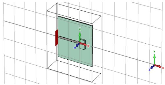
Fig. 2: Design of RDRA using double metallic strip
