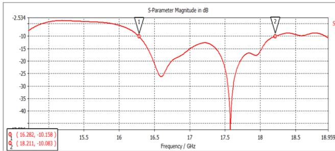
Fig.4: S-parameter result of RDRA using double metallic strip on DRA along with width
