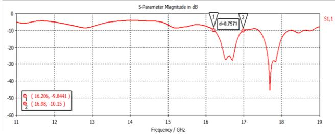
Fig. 5: S-parameter result of RDRA using double metallic strip on DRA along with length
