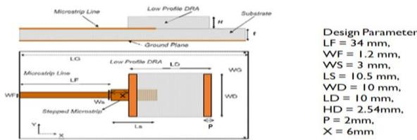
Fig. 1: Double metallic microstrip DRA (Side and Top view) [1]
