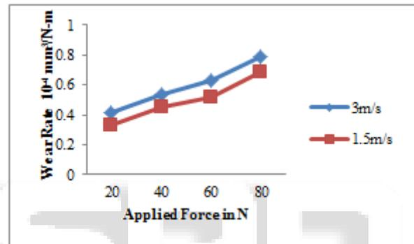
Fig. 5: Wear Rate of AA6063 SiC-Gr Hybrid composite at Different Velocity and Applied Load
