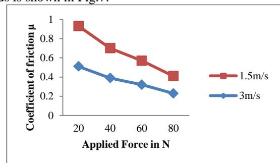
Fig.7: Coefficient Of Friction of AA6063 Sic-Gr Hybrid Composite at Different Velocity and Applied Load
