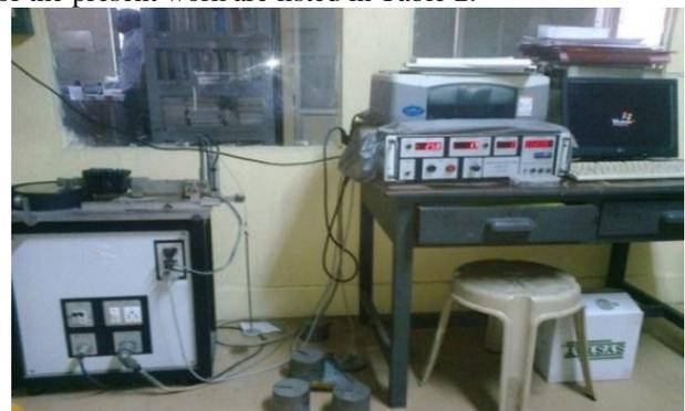
Fig. 1: Pin on Disc Apparatus
