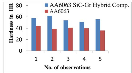
Fig. 4: Rockwell hardness of composite and AA6063
