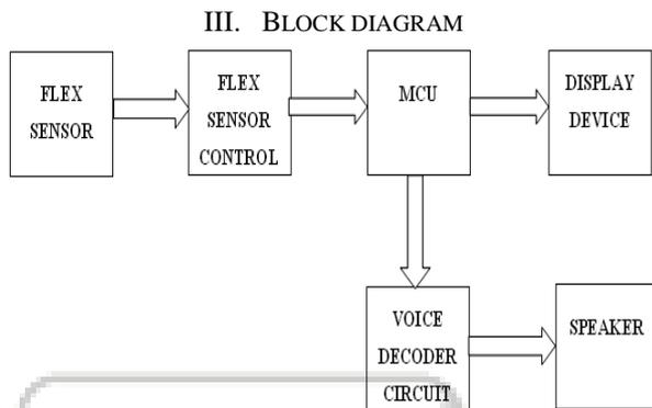
Fig. 1: Block diagram of handicap human interaction device.
