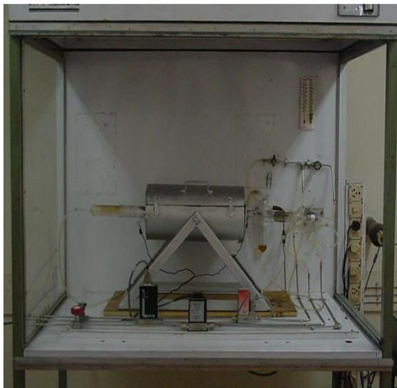
Image of CVD set-up (developed at SSPL, Delhi)
