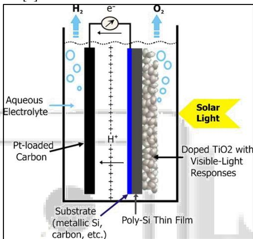
Fig. 3: schematic sketch of photo electrolytic hydrogen production. [6]
