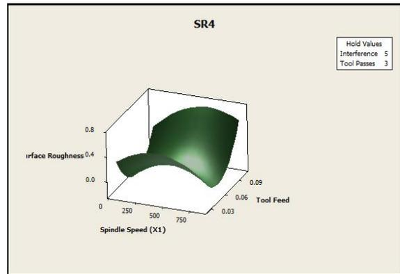
Figure 4: Effect of speed and feed on SR
