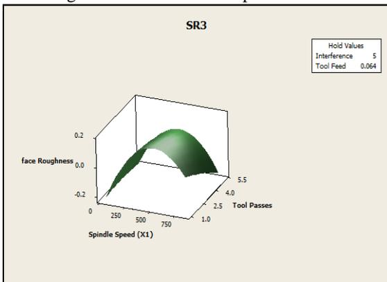
Fig. 3: Effect of speed and passes on SR
