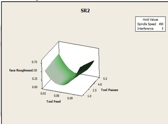
Fig. 2: Effect of feed and passes on SR
