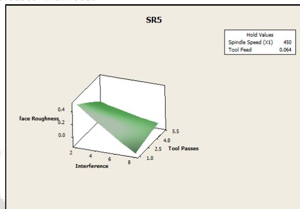
Fig. 5: Effect of interference and passes on SR
