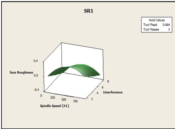
Fig. 1: Effect of speed and interference on SR
