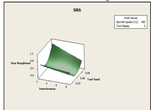
Fig. 6: Effect of interference and feed on SR
