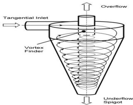
Fig. 2 Schematic view of cyclone separator
