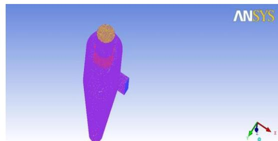
Fig. 5: Tetrahedron meshing for cyclone reactor (1.2 million elements)
