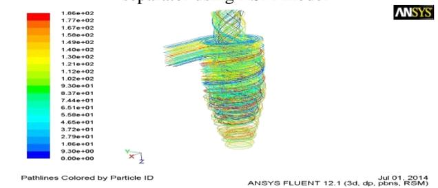
Fig. 18: Variation of particle pathlines of cyclone separator with RSM model
