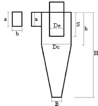
Fig. 3: Schematic view of cyclone separator
