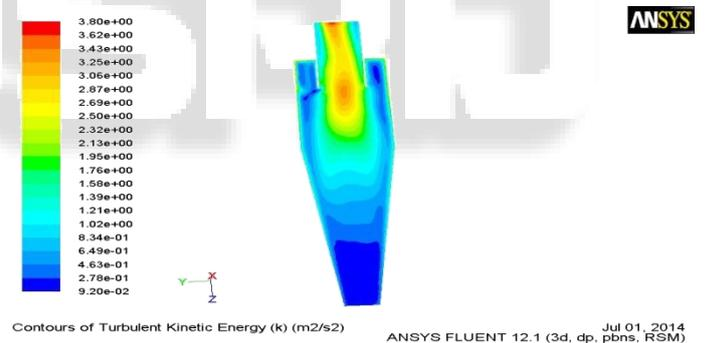
Fig. 19: Variation of turbulent kinetic energy in cyclone separator
