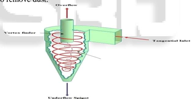
Fig. 1: Cyclone separator
