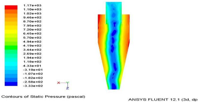
Fig. 13: Variation of static pressure in cyclone separator.
