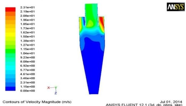
Fig. 9: Variation of velocity magnitude of cyclone separator.
