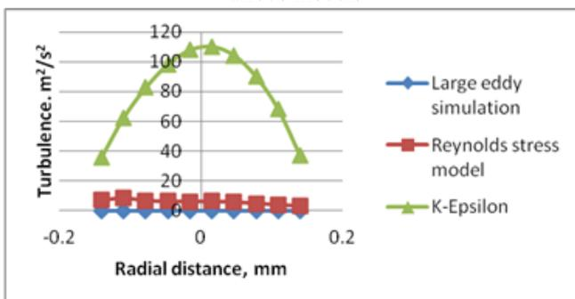
Fig. 23: Variation of turbulence with the radial distance in various models
