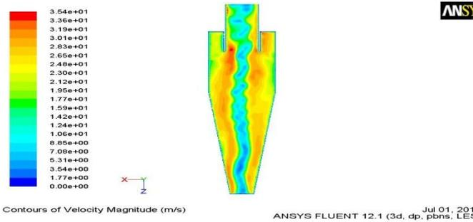
Fig. 14: Variation of velocity magnitude in cyclone separator of LES.
