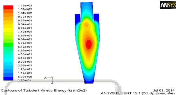
Fig. 7: Variation of turbulent kinetic energy in cyclone separator
