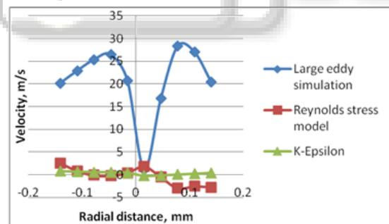
Fig. 22: Variation of velocity with the radial distance in various models
