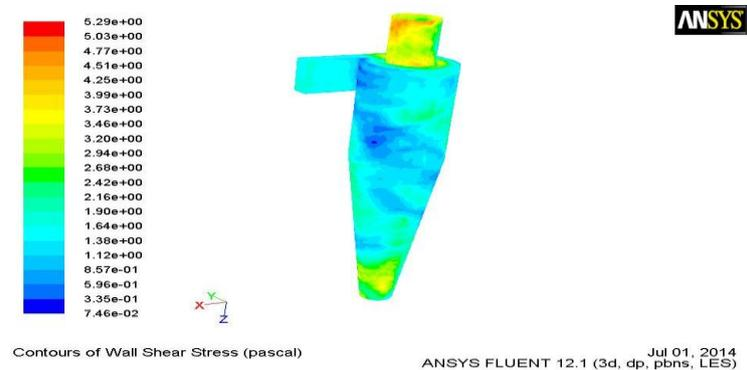
Fig. 12: Variation of wall shear stress in cyclone separator
