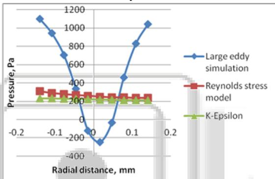
Fig. 21: Variation of pressure with the radial distance in various models
