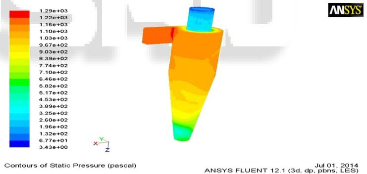
Fig. 11: Variation of static pressure in cyclone separator
