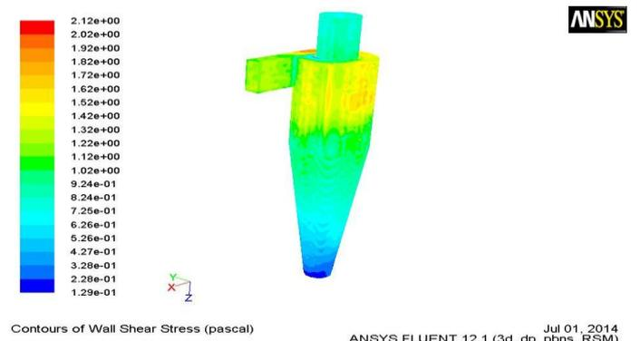
Fig. 20: Variation of wall shear stress in cyclone separator
