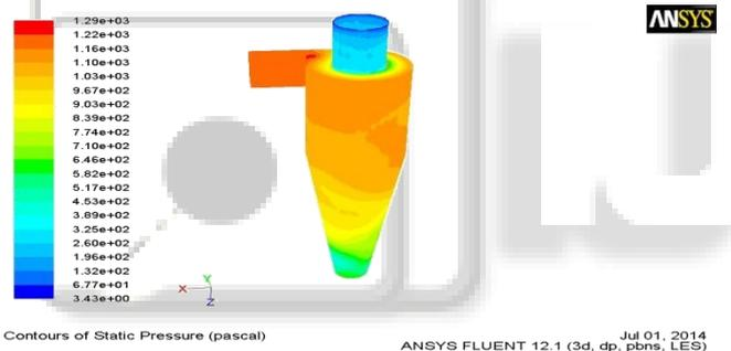
Fig. 15: Variation of maximum static pressure in cyclone separator of LES
