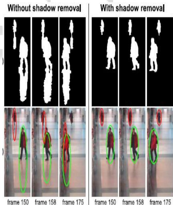
Fig. 2 (a, b): tracking trajectory in a video with and without shadow removal.
