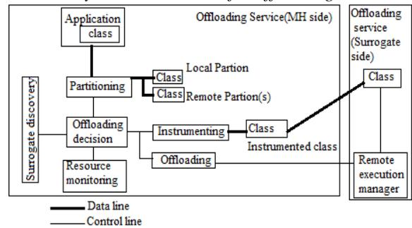
Fig. 4: System architecture
