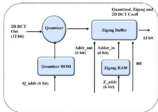
Fig. 4: Quantization & Zig-zag Architecture
