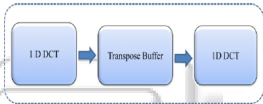
Fig. 3: 2D- DCT Process
