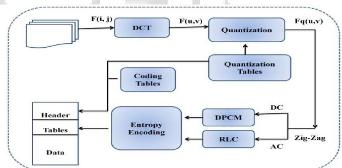
Fig. 2: Block diagram of Image compression
