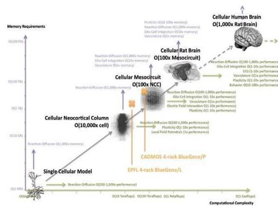
In the initial phase of its work the Blue Brain project used an IBM BlueGene/L supercomputer with 8,192 processors. Some years ago, it used a 16,384 core IBM BlueGene/P supercomputer with almost 8 times more memory than its predecessor. Today, it uses an IBM BlueGene/Q supercomputer with 65,536 cores and extended memory capabilities hosted by the Swiss National Supercomputing Center (CSCS) in Lugano.
