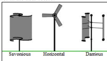
Fig 1: Types of Wind Turbine
