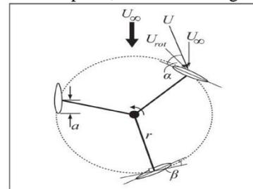
Fig 2: Plan view of turbine showing the preset blade pitch angle ( $\beta$ ), angle of attack ( $\alpha$ ), the incident wind speed due to  $U_\infty$  and rotational speed  $U_{rot}$ , and mount location offset ( $a$ ).
