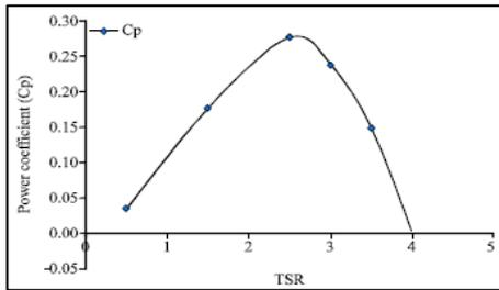
Fig 3: Performance characteristics by Cp Vs TSR graph.
