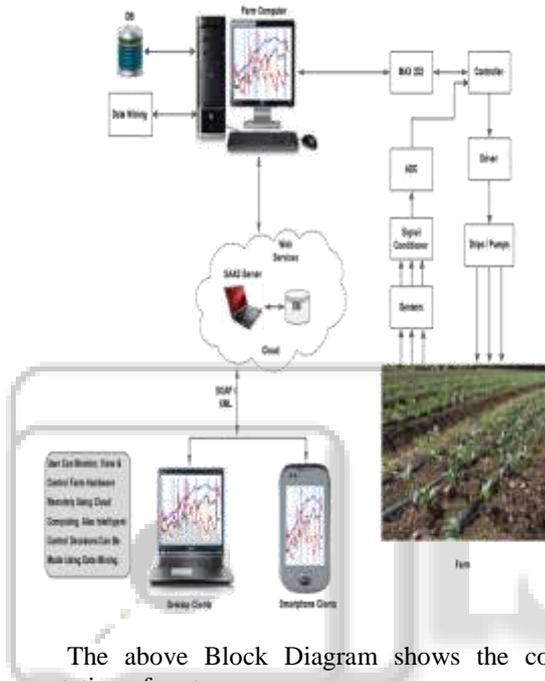
The above Block Diagram shows the complete representation of system.
