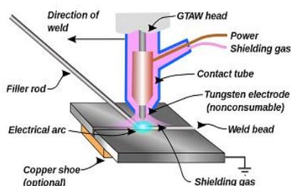
Fig. 1 Schematic Diagram of TIG welding process
