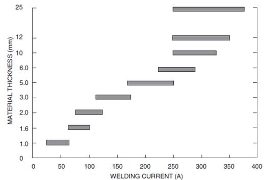
Fig. 2: Relation between material thicknesses and welding currents
