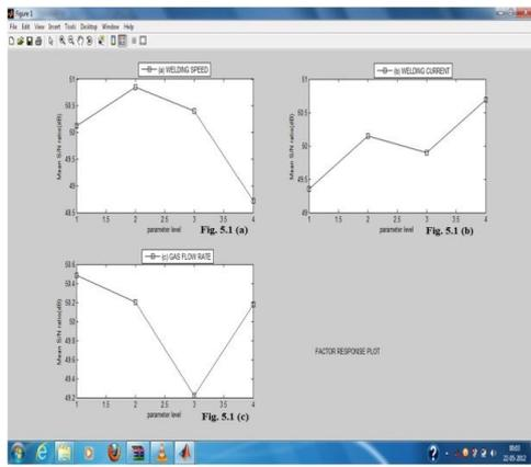
Fig 3: Factor response plot for tensile strength
