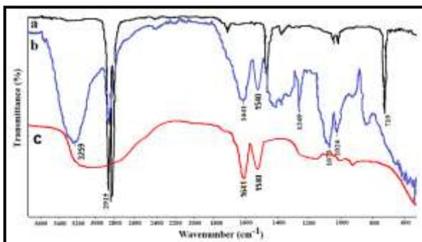
Fig. 2: FTIR spectra of latex (a), enzyme bound latex surface (b) and enzyme (c).
