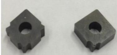
Fig. 6: Involute profile cut on Specimen1 (left) and Specimen2 (right)
