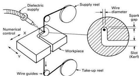
Fig. 1 Schematic Diagram of Wire EDM process
