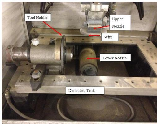
Fig. 5 Experimental Setup of the Wire EDM Machine
