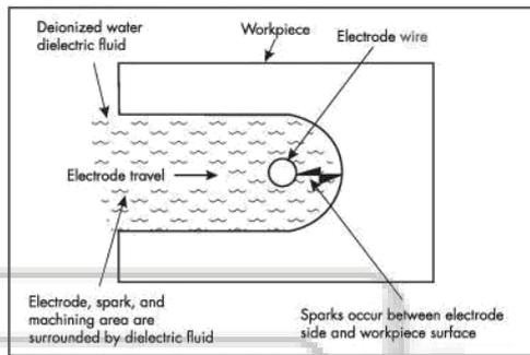
Fig. 2 Wire EDM cut with spark gap
