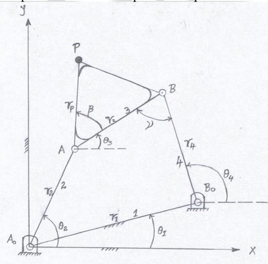
Loop-Closure equation for the four bar mechanism is
