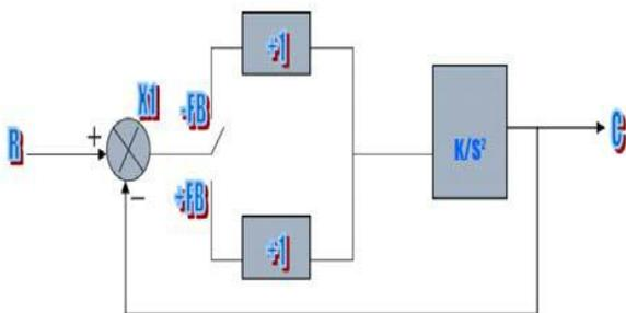
Fig. 4: Block diagram of Sliding mode control for Second order system.
