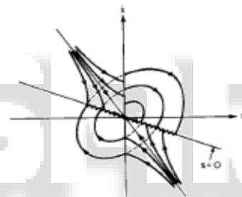
Fig. 6: sliding mode control in phase plane
