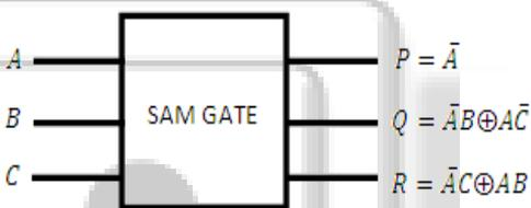
Fig. 5: Block diagram of 3x3 SAM Gate
