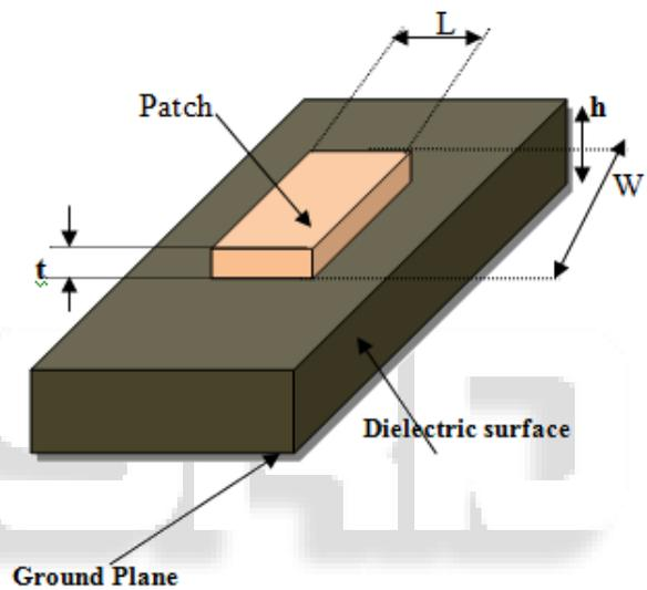
Fig. 2.1: Structure of Microstrip Antenna
