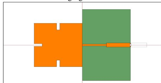
4.1 Microstrip Patch Antenna Designed using IE3D
