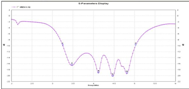
Fig. 5.2: S-parameter Plot for Reflection Coefficient v/s Frequency
