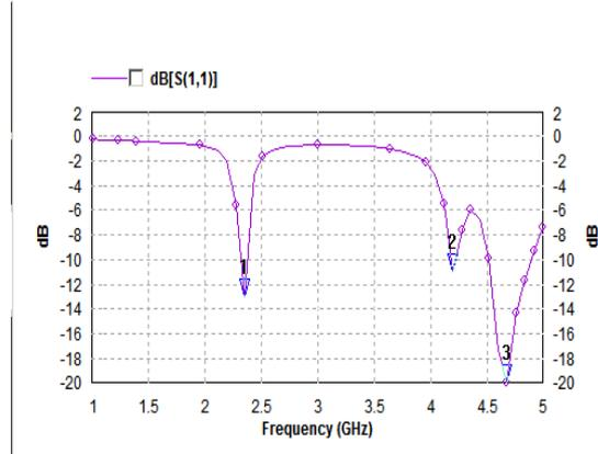
Fig. 4.2: S-parameter Plot for Reflection Coefficient v/s Frequency
