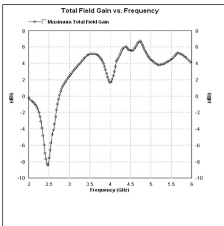
Fig. 5.8: Total Gain v/s Frequency
