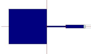
Fig. 4.1: Microstrip Patch Antenna Designed Using IE3D
