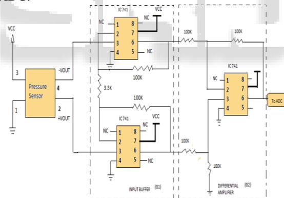
Fig. 6: Pressure Sensor
