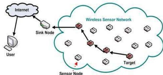
Fig. 1: Traditional Wireless Sensor Network
