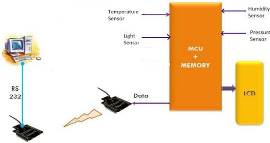
Fig. 2: Functional Block Diagram of System being Developed
