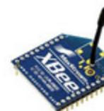
Fig. 7: Zigbee series 1 module
