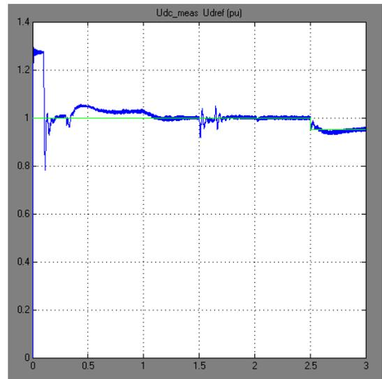
Fig. 13: DC Voltage in p.u at receiving end
