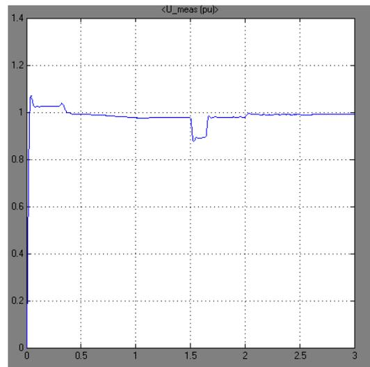
Fig. 8: Sending end AC voltage measured in p.u
