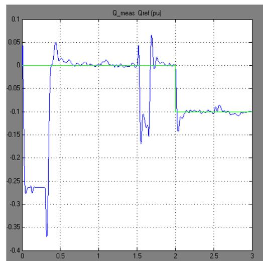
Fig.10: Reactive power in p.u at sending end
