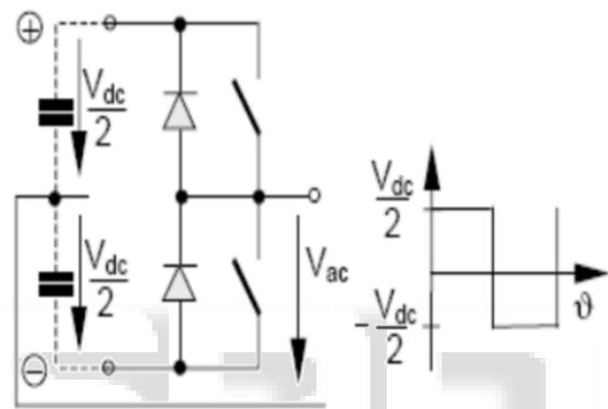
Fig. 1: Operational principle of VSC
