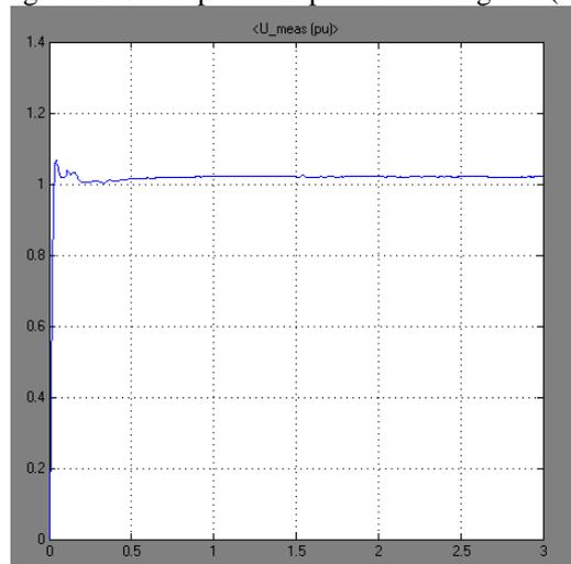
Fig. 15: Receiving end AC voltage measured in p.u
