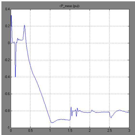
Fig. 16: active power in p.u at receiving end
