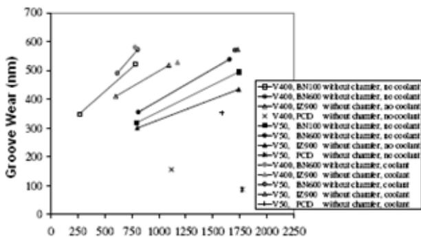
Fig. 2: Groove Wear of various PCD tools with different cutting speeds
