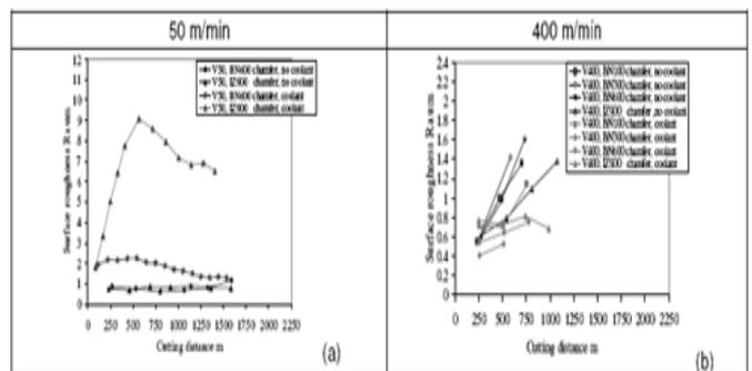
Fig. 4: cutting distance vs. Surface roughness at different speeds
