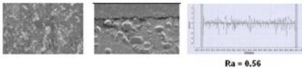
Fig. 5: SEM of machined surface roughness and its Ra value
